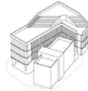
The new hospital was built around the old building. The old building continued to function during construction.
