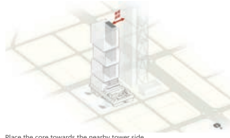
Place the core towards the nearby tower side
